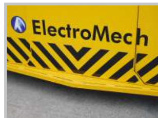
Front & Rear Safety Guard Structural safety guards at the ends to avoid collision during travel
