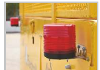
Flashing Light with Built-in Hooter Audio-visual alarm while the STC is moving
