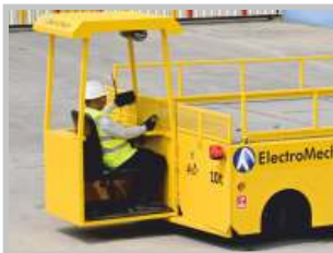
Operator's Cabin (Optional) Useful for outdoor operations and areas requiring long travelling distance
